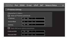
④ Go to Start → Settings → Camera → Add Camera. The DVR will automatically refresh the cameras searched. The IPC which supports the Onvif protocol may be added manually. If the IPC searched is not in the same local network as the DVR, you should select the device and click ☑ to modify the IP address.
