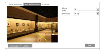
Set the alarm line number and direction. Only one line can be added. Multiple lines cannot be added simultaneously.
