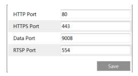
**HTTP Port**: The default HTTP port is 80. It can be changed to any port which is not occupied. **HTTPS Port**: The default HTTPS port is 443. It can be changed to any port which is not occupied.
