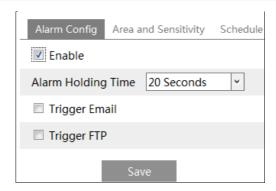
Then select the alarm holding time and set the alarm trigger options.
