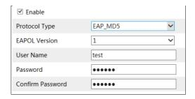
To use this function, the camera should be connected to a switch supporting 802.1x protocol. The switch can be reckoned as an authentication system to identify the device in a local network. If the camera connected to the network interface of the switch has passed the authentication of the switch, it can be accessed via the local network.
