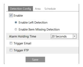
1. Enable object removal detection and then select the detection type.
