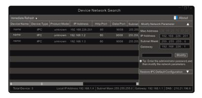
③ Modify the IP address. The default IP address of this camera is 192.168.226.201. Click the information of the camera listed in the above table to show the network information on the right hand. Modify the IP address and gateway of the camera and make sure the network address is in the same local network segment as the computer. Please modify the IP address of your device according to the practical situation.
