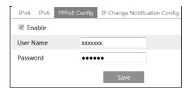
Either method of network connection can be used. If PPPoE is used to connect internet, the camera will get a dynamic WAN IP address. This IP address will change frequently. To be notified, the IP change notification function can be used.
