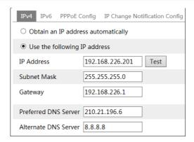
**Use IP address (take IPv4 for example)-**There are two options for IP setup: obtain an IP address automatically by DHCP protocol and use the following IP address. Please choose one of the options as needed.
