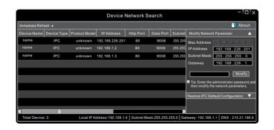
③ Modify the IP address. The default IP address of this camera is 192.168.226.201. Click the information of the camera listed in the above table to show the network information on the right hand. Modify the IP address and gateway of the camera and make sure the network address is in the same local network segment as that of the computer. Please modify the IP address of your device according to the practical situation.
