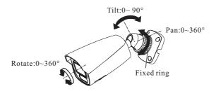
6 Tighten the fixed ring to finish the installation.
