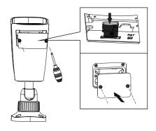
② Drill the screw holes and the cable hole (if you want to route through the ceiling) on the wall or ceiling according to the drill template.
