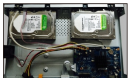
③ Place the HDDs onto the bottom of the case.
