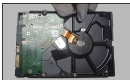
② Screw the screws into the holes of HDD but not tighten them.
