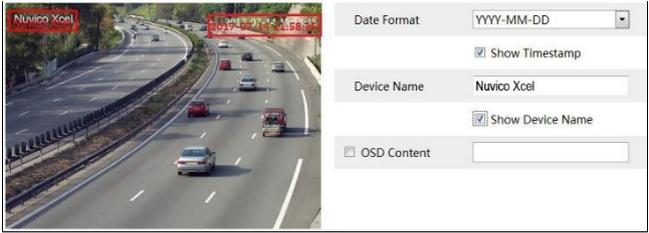
Time stamp, device name and OSD can be set up here. After enabling the corresponding display and entering the content, drag them to change their position. Then press the “Save” button to save the settings.
