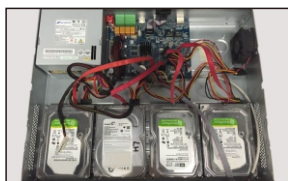
⑤ Connect the power and data cables.
