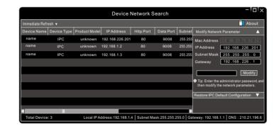
3 Modify the IP address. The default IP address of this camera is 192.168.226.201. Click the information of the camera listed in the above table to show the network information on the right hand. Modify the IP address and gateway of the camera and make sure its network address is in the same local network segment as that of the computer. Please modify the IP address of your device according to the practical situation.
