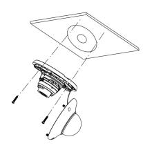
5 Three-axis adjustment. Before adjustment, preview the image of the camera on a monitor and then adjust the camera according to the figure below to get an optimum angle.
